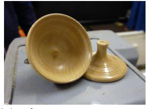
John then placed a sycamore blank in the chuck and started turning the base of a top.
